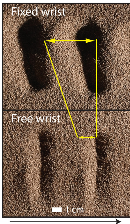
Figure 6. Tracks of FBot in poppy seeds for fixed and free wrist configurations with \theta_f = 45^\circ and \psi_f = 0 (the black arrow indicates direction of robot motion). The vertical yellow line marks the location of initial flipper insertion, while left arrowheads mark visible extent of disturbed ground which, for the fixed wrist, is significantly larger and extends into the track from the previous step.
