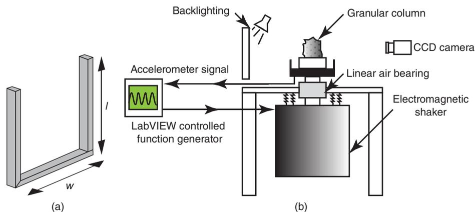
**Figure 17.3** Relaxation dynamics of U-particle columns are studied through a mechanical vibration experiment. (a) U-Particle geometry. Width,  $w$ , is held constant and length,  $l$ , is varied. (b) A computer-controlled shaker table applies sinusoidal forcing to a granular column. A high-speed camera records column collapse from the side.
