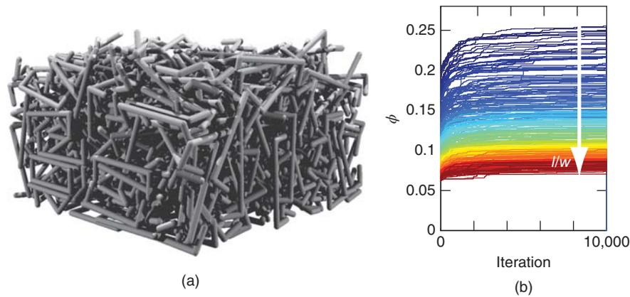
**Figure 17.8** Computer simulated u-particle ensembles. (a) A computer-generated ensemble of u-particles of  $l/w = 0.35$ . (b) Volume fraction of particle ensembles as a function of simulation iteration. Particle ensembles are packed together in a Monte Carlo simulation until the volume fraction reaches a steady-state. Particle  $l/w$  is varied from 0 to 1.4 with increasing  $l/w$  indicated by arrow.
