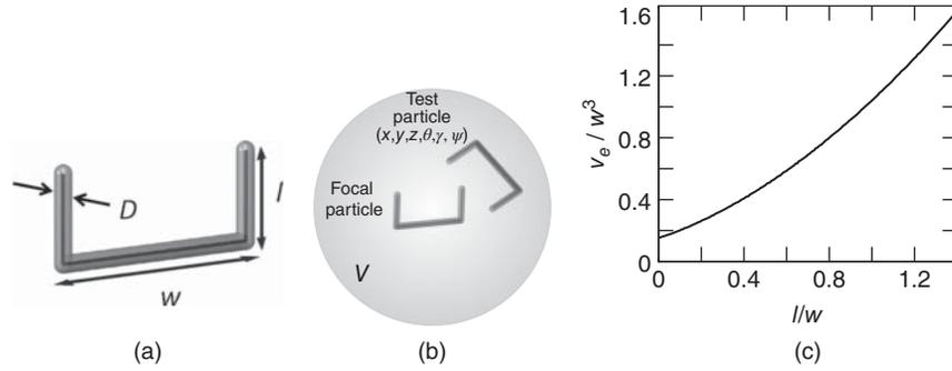
**Figure 17.7** Overview of simulation. (a) Three spherocylinders form a u-particle in computer simulation with dimensions given in the text. (b) We compute the excluded volume of u-particles through a Monte Carlo simulation measuring the probability for two randomly placed particles to overlap within a large volume  $V$ . (c) Excluded volume of u-particles as a function of  $l/w$ .
