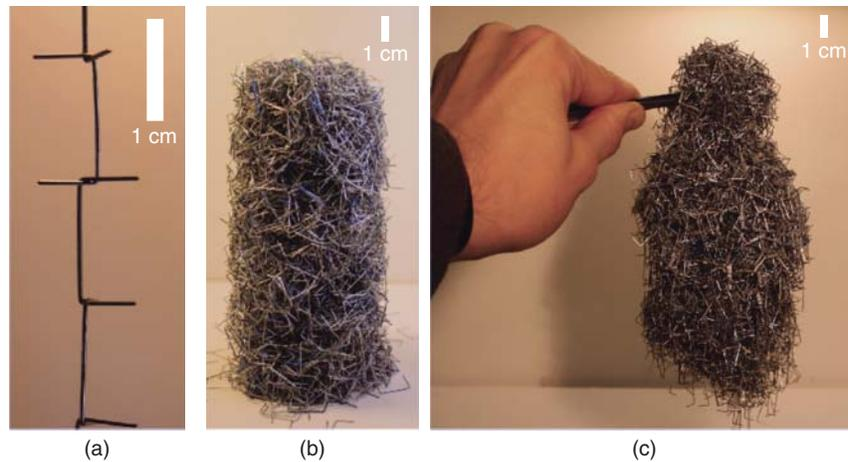
**Figure 17.2** u-Particle assemblies. (a) u-Particles interpenetrate to support tensile loading. (b) A free-standing column of entangled u-particles. (c) Grasping the tower with tweezers illustrates the tensile strength of this granular assembly.
