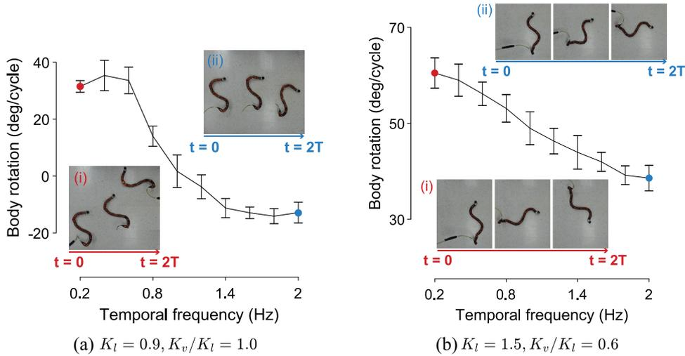
**Fig. 7.** Temporal frequency dependency of unstable gaits. Dependence of the rotation angle (per cycle) on the temporal frequency of (a) statically unstable translational sidewinding gaits and (b) statically unstable rotational sidewinding gaits on SEA robot experiments. The subplots (i) and (ii) show the snapshots of the SEA robot implementing gaits in low temporal frequency (0.2 Hz, red) and high temporal frequency (2.0 Hz, blue) over three gait cycles.
