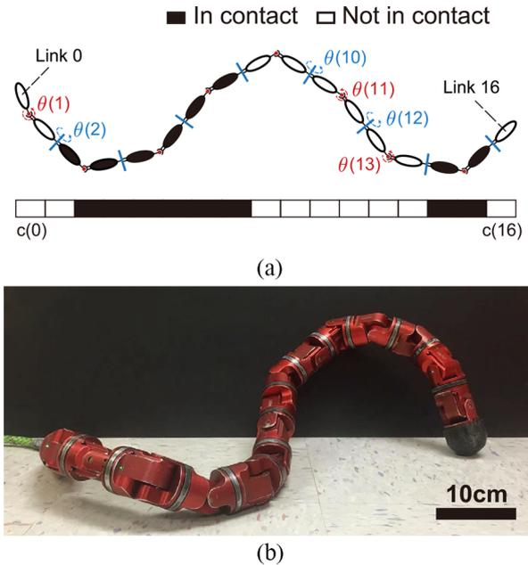
**Fig. 1.** Theoretical model and experimental robot. (a) The theoretical model for the sidwinder robots. The filled black ovals indicate the ground contact phase whereas the white ovals indicate a no ground contact phase. The contact state is labeled in black ( $c(i)$ ). The joint angle in blue indicates pitch joints and the joint angle in red indicates yaw joints. (b) The SEA robot used to test the effectiveness of our stabilization approach.
