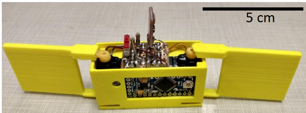
Figure 9.12: Assembled flat smarticle front view
