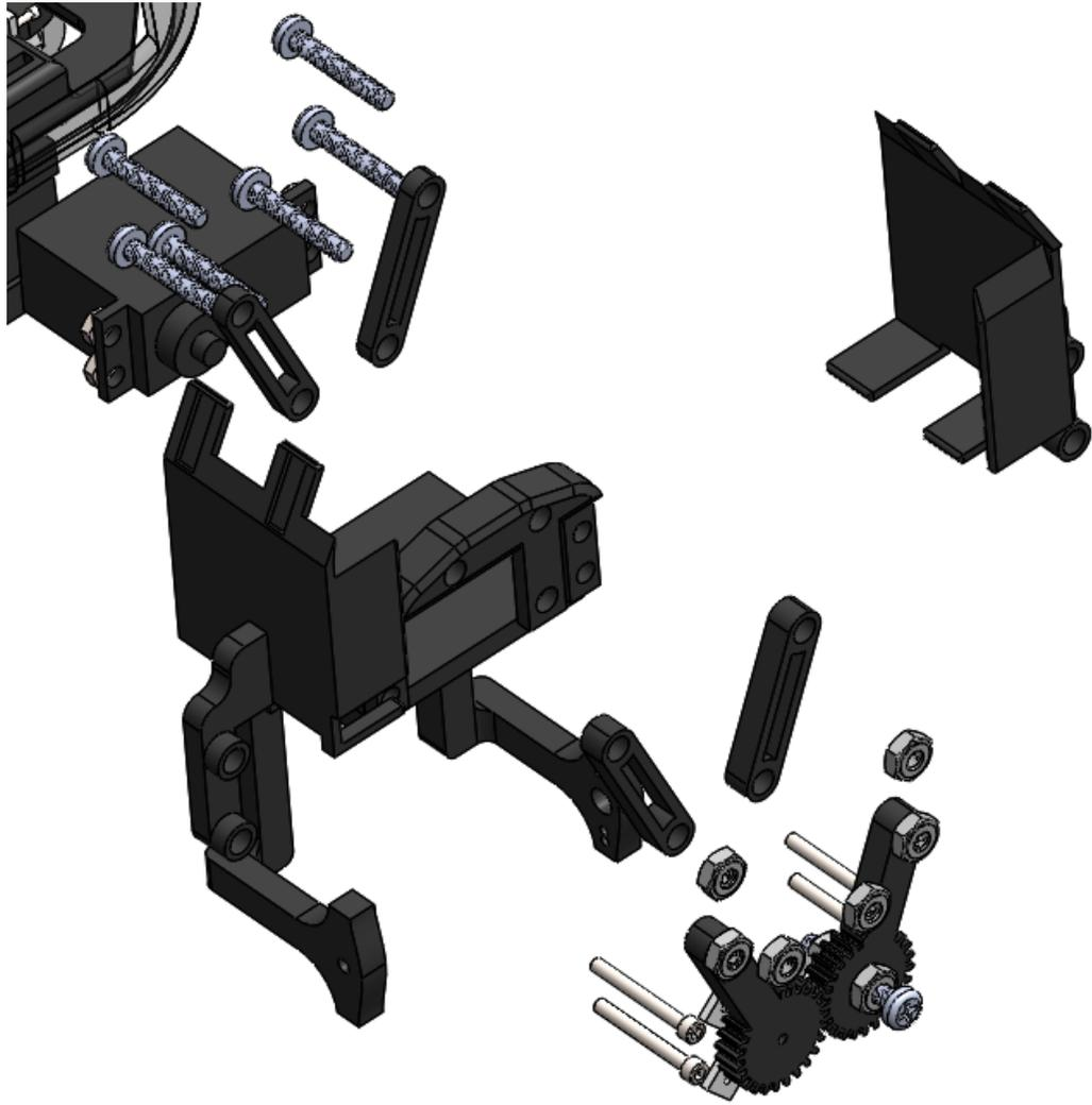
Figure 4.6: Exploded view of gripper assembly
