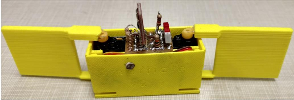
Figure 9.13: Assembled flat smarticle back view
