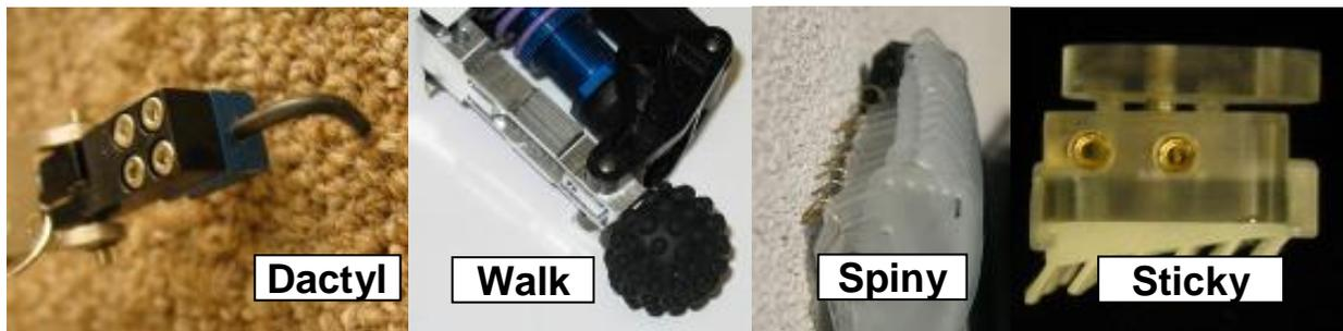
**Figure 10: Photographs of four different types of feet used on the RiSE platform.**
