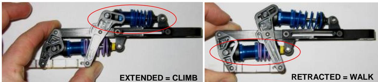
**Figure 8: The new compliant leg structure designed to enable independent tuning of extension and compression compliance as well as damping.**
