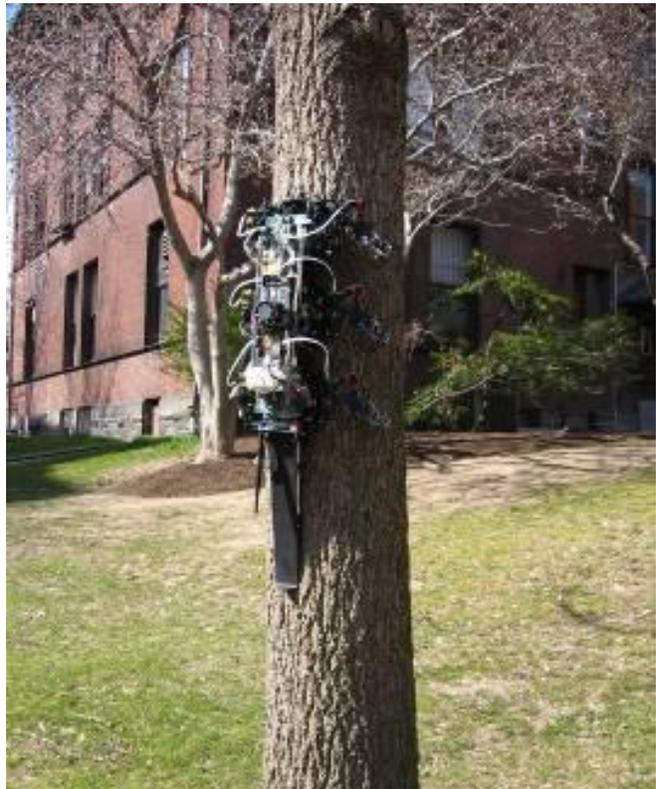
**Figure 1: The RiSE robot climbing a tree.**
