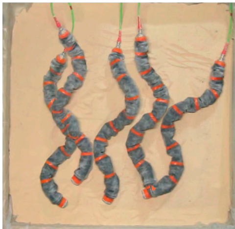
Movie S4. The snake robot performing reversal turning in a sand bed due to a 180^\circ phase shift in the vertical wave.
