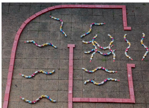
Movie S6. The snake robot (at 3x speed) navigating a trackway using the three turn types described in this paper.
