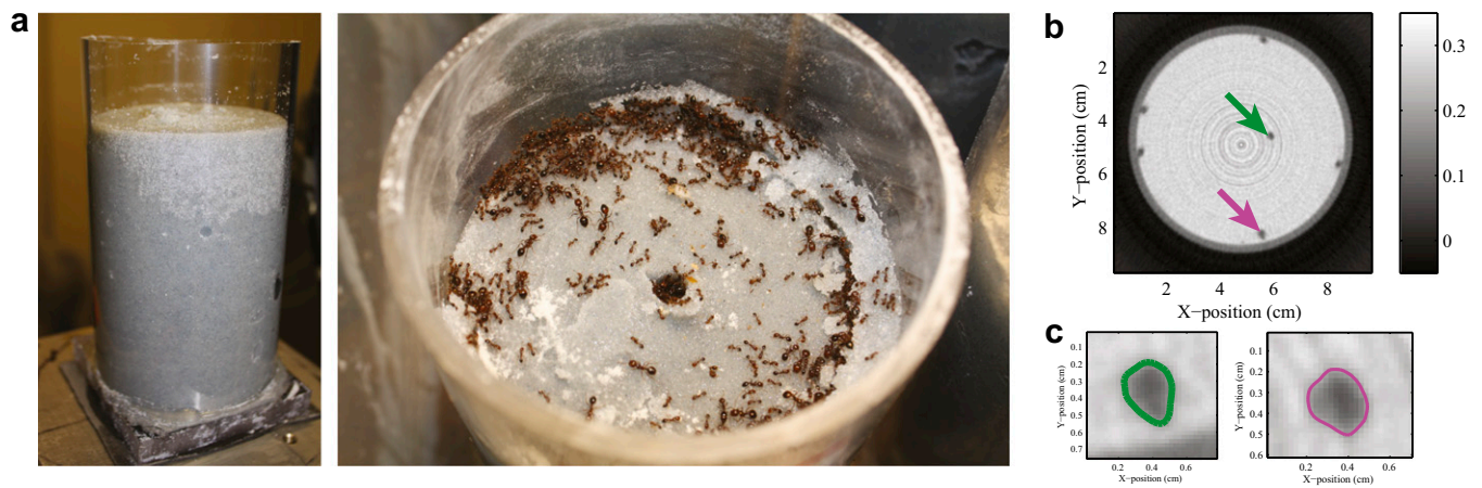
Fig. S1. Overview of the X-ray CT digging trials. (A) Digging arena consisted of a circular plastic, or aluminum container of diameters 8.2 or 3.8 cm, filled to a height of ~12–15 cm with a simulated soil of monodisperse 50, 210, or 595 \mu\text{m} diameter, wetted, glass beads. 8.2 cm diameter container shown in left and right images of (A). (B) A horizontal cross-section from X-ray CT reconstruction at a depth of 6.8 cm from the surface. Top and bottom arrow indicate two tunnels not adjacent to arena wall. Four other tunnels are present but against the tunnel wall. (C) Cross-section of the top ( Left ) and bottom ( Right ) tunnels from B with extracted tunnel shape from active contours method shown as green ( Left ) and purple ( Right ) lines.
