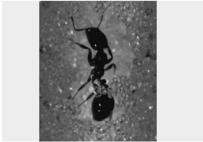
Movie S2. Rapid ascent in ant-constructed tunnel. The substrate consists of wetted 250 micron approximately spherical glass particles. During the middle of the climb, ant slips and falls backward but its motion is rapidly arrested.
