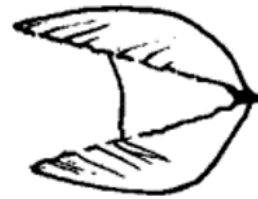
Figure 1.7: Scallop Theorem. In high Reynolds number fluids, a scallop can leverage inertia with a single degree of freedom to produce motion. In low Reynolds, inertial terms in the Navier-Stokes equation are negligible and propulsion is not achieved with symmetric gaits (in shape or time). Figure from [72].
