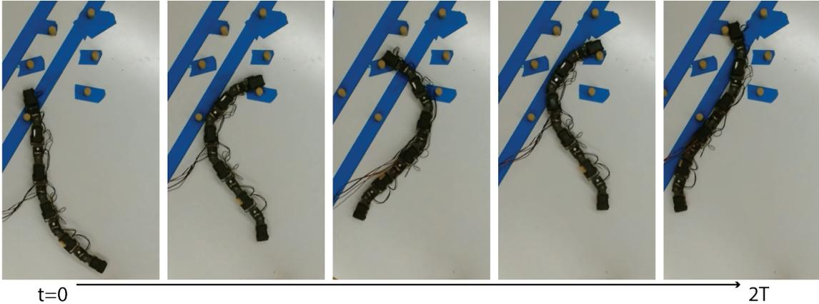
Figure 2.40: **Unevenly distributed post experiments** A sequence of video frames of the robot executing the elliptical-wave gait in an unevenly arranged planar peg board over two gait cycles.
