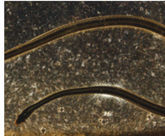
Figure 7. It is difficult to see the pattern of a snake adjusting its weight as it slithers, because the snake's body is often in contact with the ground. One way to visualize regions of higher applied force is to film a snake slithering on gelatin, illuminated from below, between cross-polarizing filters ( left ). The orientation of the filters initially blocks the polarized light from reaching the imager, but when the snake pushes on the gelatin, the light is rotated and can be detected by the camera, as shown by the luminous regions ( middle and right ). Although the adhesiveness of the gelatin can interfere with the snake's natural locomotion, this technique suggests that less of the snake may be in contact with the ground than was previously believed.
