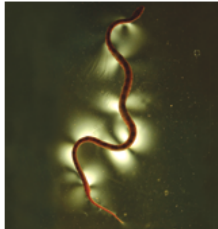
Figure 7. It is difficult to see the pattern of a snake adjusting its weight as it slithers, because the snake's body is often in contact with the ground. One way to visualize regions of higher applied force is to film a snake slithering on gelatin, illuminated from below, between cross-polarizing filters ( left ). The orientation of the filters initially blocks the polarized light from reaching the imager, but when the snake pushes on the gelatin, the light is rotated and can be detected by the camera, as shown by the luminous regions ( middle and right ). Although the adhesiveness of the gelatin can interfere with the snake's natural locomotion, this technique suggests that less of the snake may be in contact with the ground than was previously believed.
