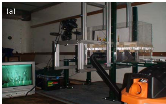
Figure S3: (a) Field apparatus including trackway, cameras and blowers was housed in a truck. (b) Fluidized bed trackway and high speed cameras.
