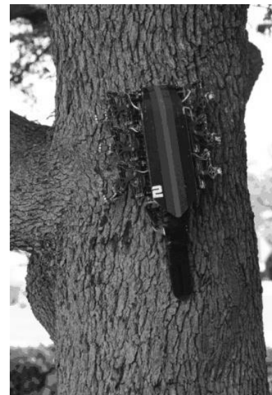
Figure 4. The RiSE Platform ascending a tree
