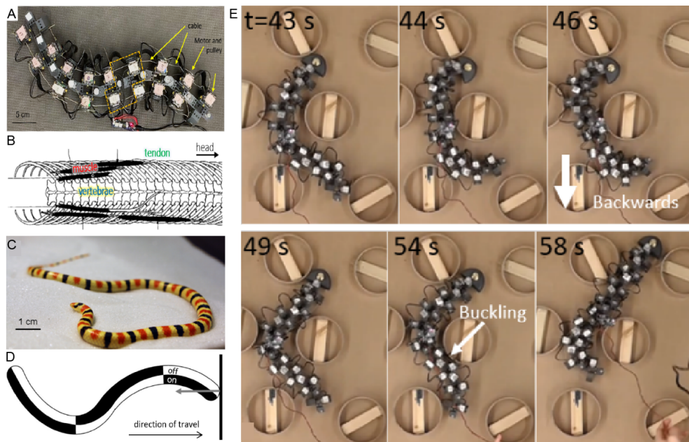
Figure 1.5: Embodied intelligence via muscle-like actuation. (A) Robophysical snake model that uses tendons to actuate the body undulation [42]. (B) Simplified snake anatomy showcasing the musculoskeletal system that drives lateral body bending in snakes. (C) C. occipitalis on model desert sand. (D) Cartoon depicting muscle activation and compliance. (E) Snapshots of robot demonstrating passive buckling and reversals to traverse a cluttered lattice.
