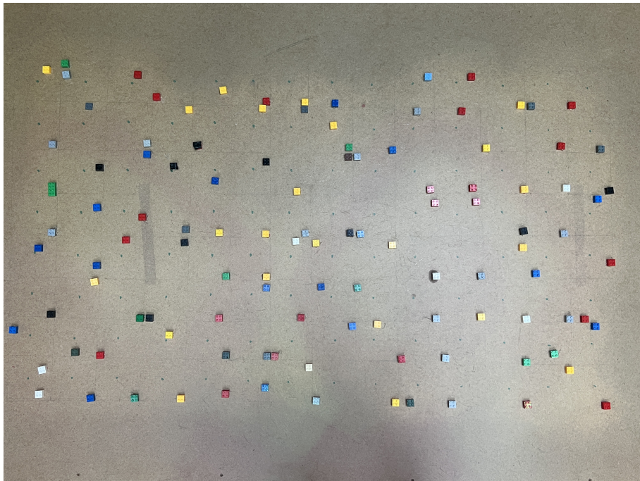
Fig. S3. Lego field: 120 Lego bricks(1.5cm × 1.5cm × 1cm) were randomly placed in an 150cm × 90cm area. Their distribution was generated by uniformly distribution.
