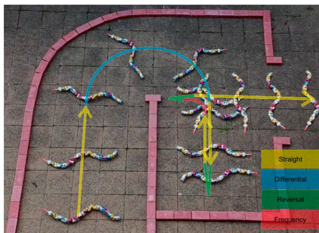
**Fig. 6.** Images from [Movie S6](#) showing the sidewinder robot moving through a trackway using three turn types (labeled) and straight-line side-winding. The size of the test course is 3 × 3 m<sup>2</sup> and the robot completed the course in 48 s.
